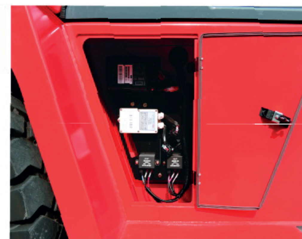
Independent integrated electric cabinet
